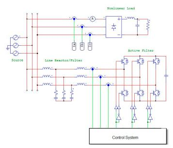
Fig 20: Parallel active filter schematic and connection
