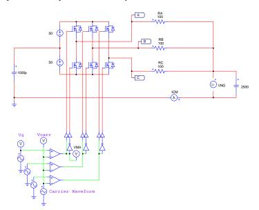
Figure 36: Simplified circuit for common mode shift
