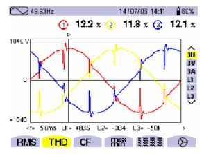
Fig 28 : 3 x 900HP DC drives voltage waveforms with 3% AC line reactors only
