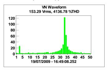
Fig 41: Phase V1 to ground voltage harmonic spectrum (V) when draw-works or top drive VFDs are assigned or running
