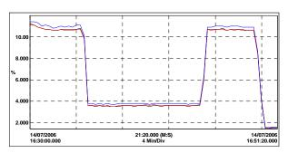
Fig 22: Uthd on 3 x 900HP/600kW DC drives without/with/without parallel broadband active harmonic filter.
