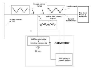
Fig 19: Parallel active filter current waveforms
