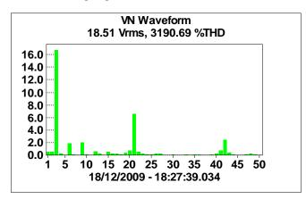
Fig 42: Phase 1 to ground voltages on EMC compliant VFD drilling package. Note - two VFDs systems running.
