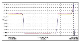
Fig 21: Ithd on 3 x 900HP/630kW DC SCR drives without/with/without parallel broadband active filter.
