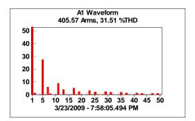
Fig 10 : DC SCR with line reactor. Typical harmonic current spectrum (%)
