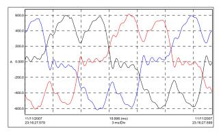
Fig 6: Example of 1500HP (1100kW) VFD phase currents at moderate load. 34.88% Ithd.
