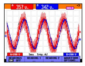
Fig 40: Red trace represents Phase V1 to ground voltage when the draw-works and/or top drive is assigned or running
