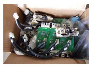
Fig 31 : Damage due to voltage spikes on small to medium powered VFDs. Failure of rectifier devices and DC bus capacitors
