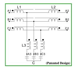
Fig 13 – Advanced wide spectrum filter schematic.
