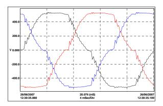
Fig 3 : Example of line voltages distorted by AC VFDs (8.8% Uthd) .
