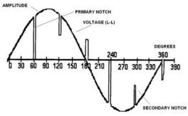
Fig 24: Primary and secondary line notching
