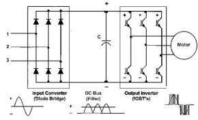
Fig 4: Simplified 6 pulse AC VFD schematic
