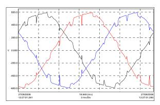
Fig 27 : 900HP DC drive line voltages with wide spectrum filter T type. Note - 1 x 700HP/500kW and 1 x 400HP/315kW untreated DC drives on same supply
