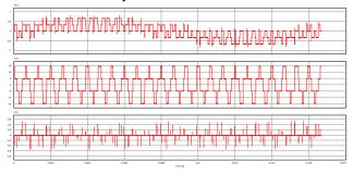
Figure 38: Top: Motor Drive Line to neutral voltage Middle: Neutral to ground voltage Bottom: ICM ground return current. All waveforms are shown with parasitic capacitance connected
