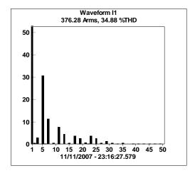
Fig 7 : Example of 1500HP (1100kW) VFD current harmonic spectrum (%). (Fundamental rescaled to 50% to show detail. Partial resonance at 23<sup>rd</sup> and 25<sup>th</sup> harmonic)
