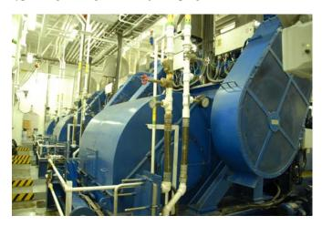
Fig 1: Mud pumps controlled by adjustable speed drives
