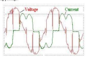
Fig 26: Severe line notching on due to fully controlled SCR rectifiers on DC drilling package
