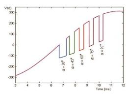
Fig 32: Notch depth variations on firing angle changes
