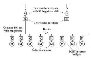
Fig 8 : Common DC bus system with quasi 12 pulse harmonic mitigation configuration
