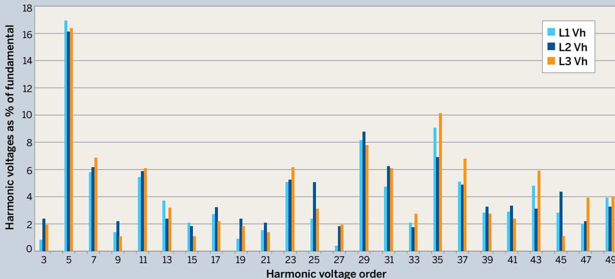
**Illustrates an installation where the THDv measured on a 690V drilling package was 27.1% (18.9% above the 21st order, due to the use of a number of 24-pulse variable frequency drives). The recommended THDv limit was 5%.**
