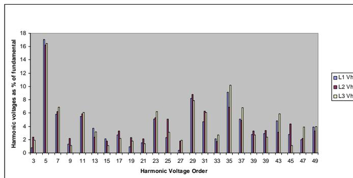
Fig 11 - Offshore oil platform harmonic voltage spectrum measured on 690V drilling package
