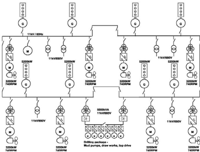
Fig 2 : Typical DP3 semi-submersible drilling rig
