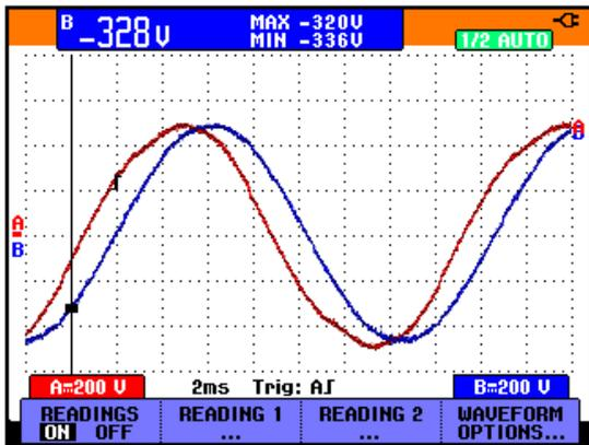
Fig 39 : Red trace represents typical Phase V1 to ground voltage when neither the draw-works and/or top drive VFDs are assigned or running
