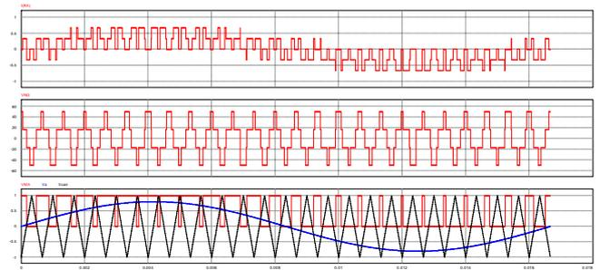
Figure 37 : Top: Motor Drive Line to neutral voltage Middle: Neutral to ground voltage Bottom: IGBT modulation on phase A, all waveforms are shown without parasitic capacitance connected
