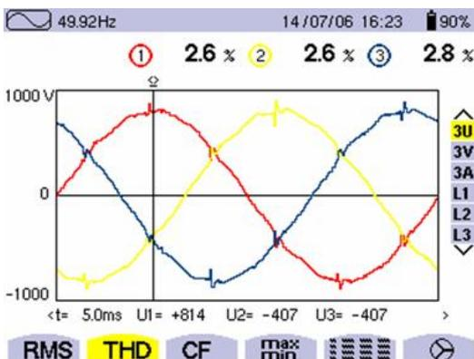
Fig 29 : 3 x 900HP DC drives voltage waveforms with active harmonic filter and 3% AC line reactors.
