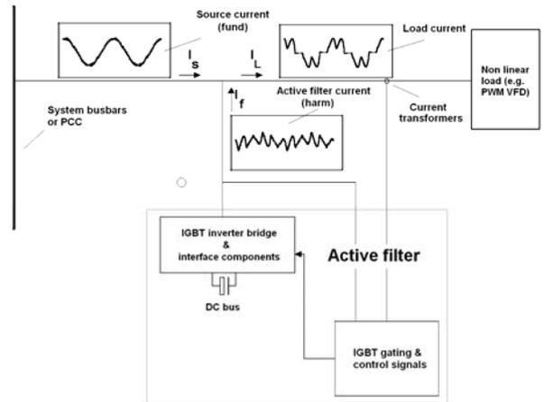
Fig 19 : Parallel active filter current waveforms
