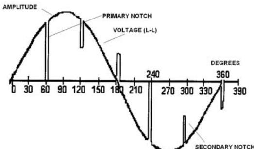
Fig 24 : Primary and secondary line notching
