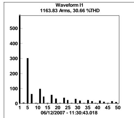
Fig 16 – 900HP/630kW DC SCR drive harmonic current spectrum. No mitigation – 30.66% Ithd
