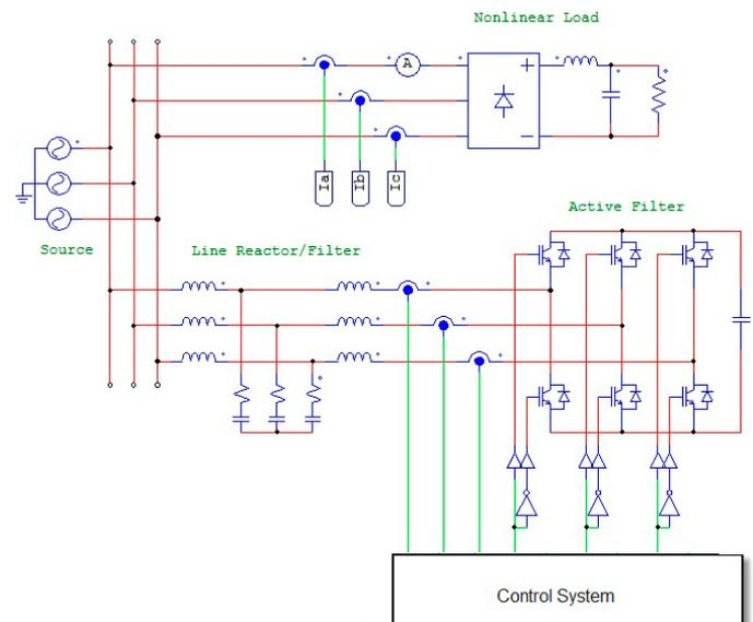
Fig 20: Parallel active filter schematic and connection
