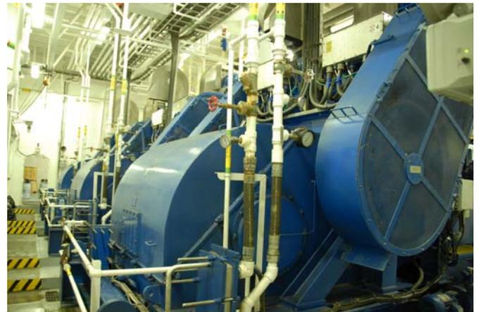
Fig 1 : Mud pumps controlled by adjustable speed drives
