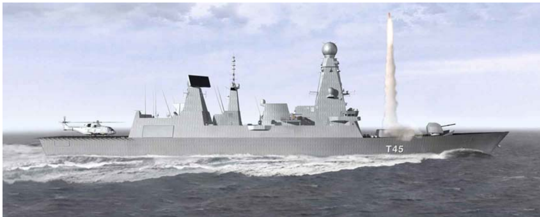
Fig 21 – UK Type 45 destroyers with 2 x 20MW PWM VFDs for propulsion (Navy News)
