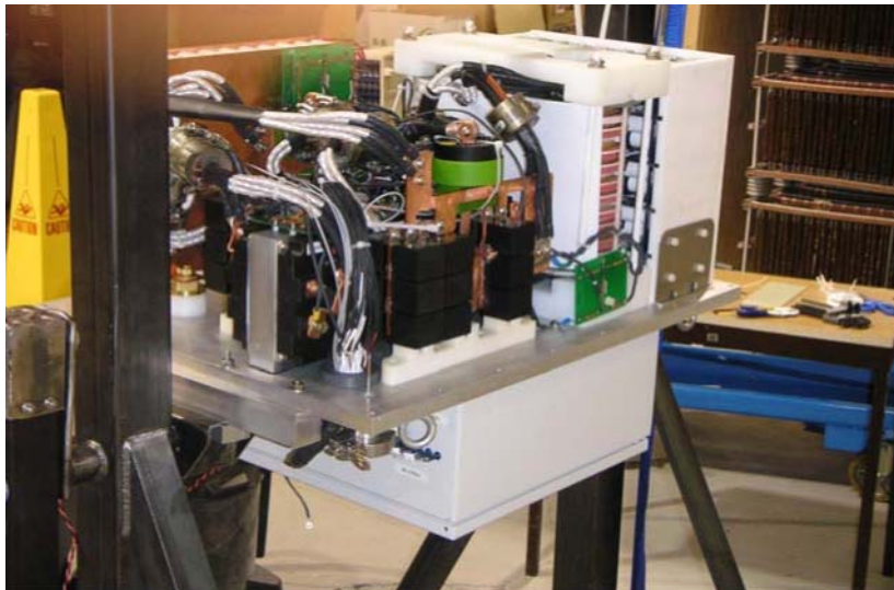
Fig 8 - 250kW AC-Link™ AC-DC converter for 480VAC-50kVDC. The integral high frequency transformer weighs 11kg.
