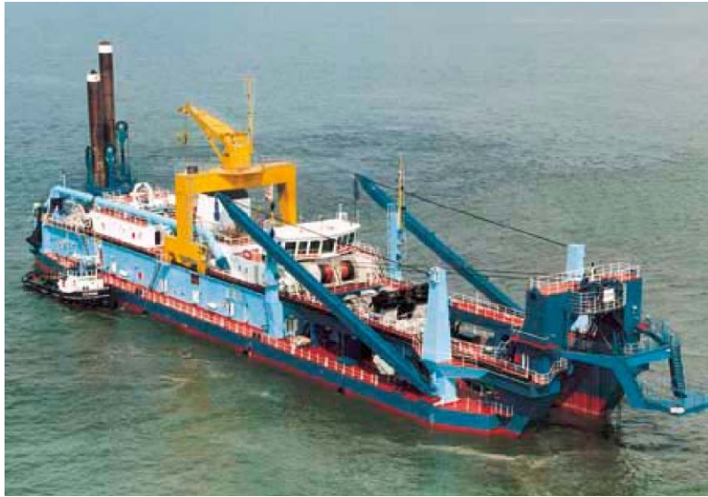
Fig 32 – Example of a cutter dredger with VFDs propulsion and other duties (Bakker Sliedrecht)
