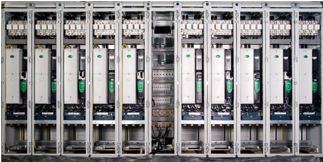
Fig 25 – Typical common DC bus system with PWM IGBT output modules fed from a common rectifier and DC capacitor based bus (Control Techniques)
