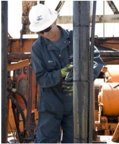
Fig 29 – Electrical submersible pump been fed into the ‘hole’ (Centrilift)
