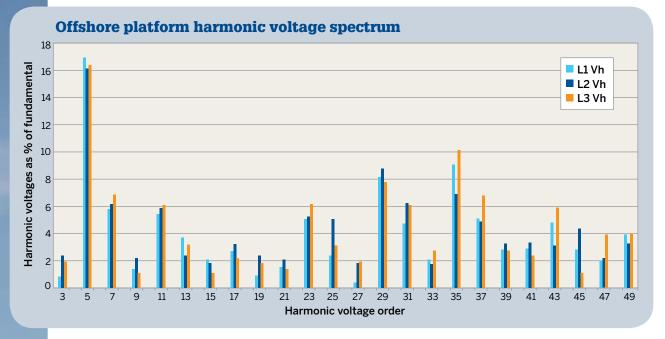
Illustrates an installation where the THDv measured on a 690V drilling package was 27.1% (18.9% above the 21st order, due to the use of a number of 24-pulse variable frequency drives). The recommended THDv limit was 5%. Source: Harmionic Solutions.
